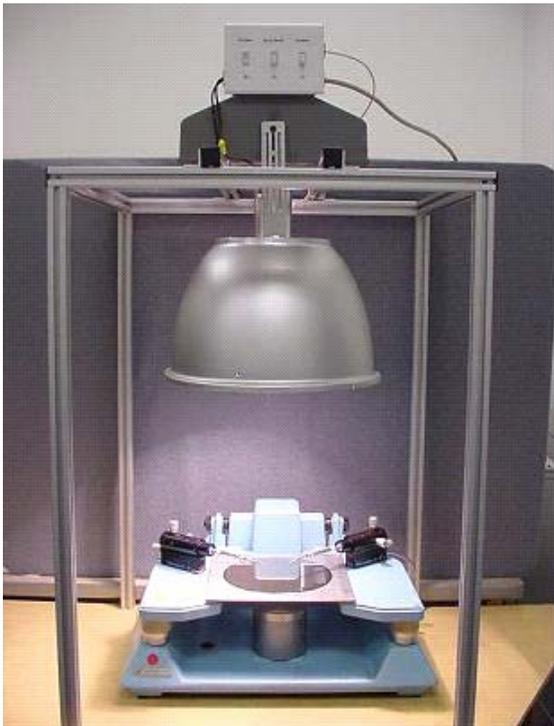
**Figure 5. The Solar Cell Prober/Solar Simulator**
