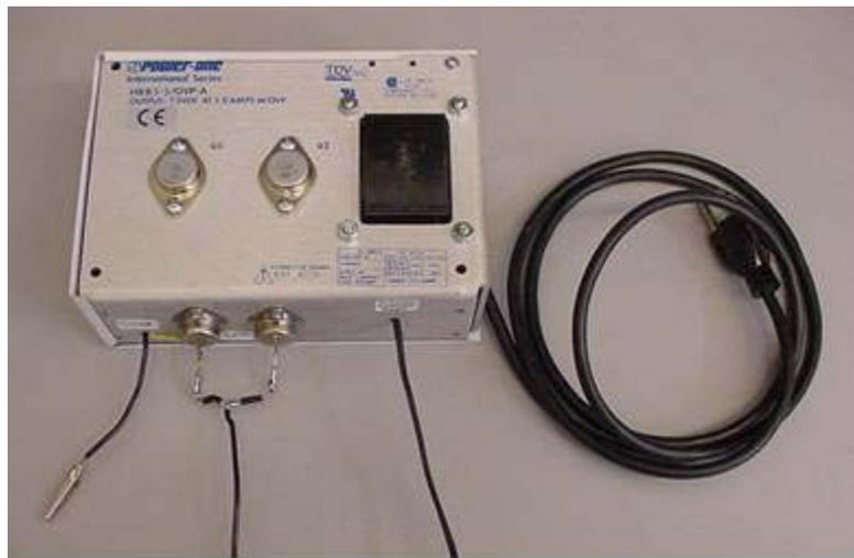
**Figure 3. Photograph of the High Current Buffer Amplifier**
