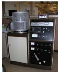
Vacuum Deposition System used in Al vapor deposition.
