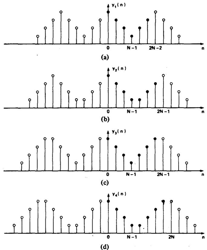
Fig. 2. Four different periodic even extensions of the nonzero  $x(n)$  samples in Fig. 1(a). (a)  $y_1(n)$  is a  $(2N-2)$ -point even extension. (b) and (c)  $y_2(n)$  and  $y_3(n)$  are two different  $(2N-1)$ -point even extensions. (d)  $y_4(n)$  is a  $2N$ -point even extension. The DCT discussed in this paper is derived from the  $2N$ -point even extension  $y_4(n)$ .
