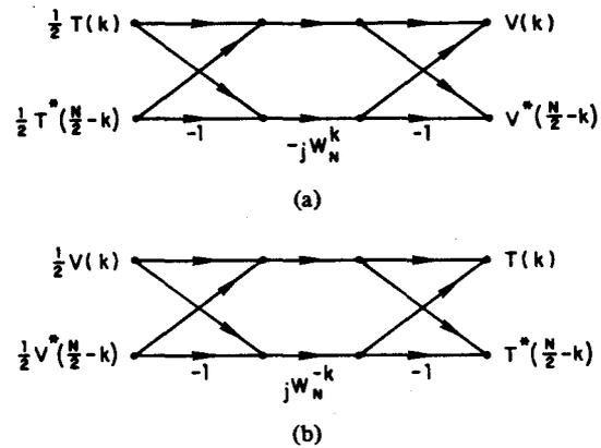
Fig. 5. (a) Supplementary flowgraph for computing the FFT of a real sequence. The computation in the figure is performed for  $0 \leq k < [N/4]$ . (b) Supplementary flowgraph for computing the IFFT of a Hermitian symmetric sequence. The computation is performed for  $0 \leq k < [N/4]$ .
