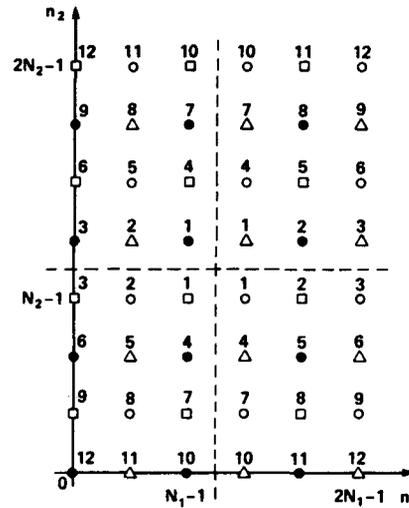
Fig. 4. An example of a 2-D  $(N_1 \times N_2)$ -point sequence and its  $(2N_1 \times 2N_2)$ -point even extension. Here,  $N_1 = 3$  and  $N_2 = 4$ . The sample values are given numerically in the figure. The four sequences defined in (39) in the text are indicated in the figure as follows: filled circles,  $v(n_1, n_2)$ ; triangles,  $w_1(n_1, n_2)$ ; squares,  $w_2(n_1, n_2)$ ; open circles,  $w_3(n_1, n_2)$ .
